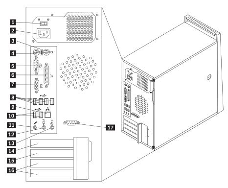
Figure 2. Rear connector locations
